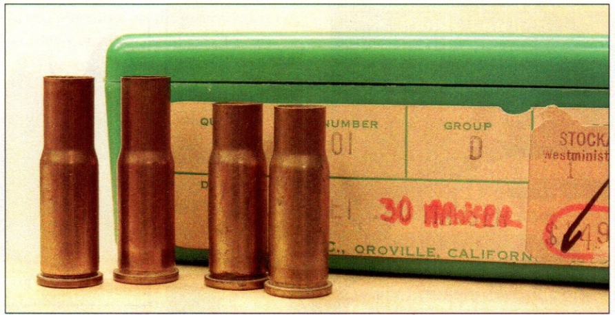
Little wildcat rounds from the 1960s included the 38 Special and 357 Magnum cases formed in 30 Mauer or 30 Luger full-length sizing dies.
