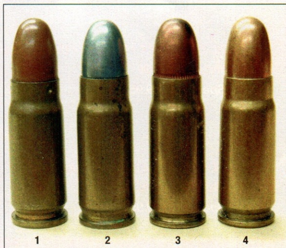
Ancestors of the 30 Luger are the: (1) 7.65mm Mannlicher, (2) 7.65mm Borchardt, (3) 7.63mm Mauser and (4) 7.62mm Tokarev. All are the same physical size, but loaded to different pressures.
