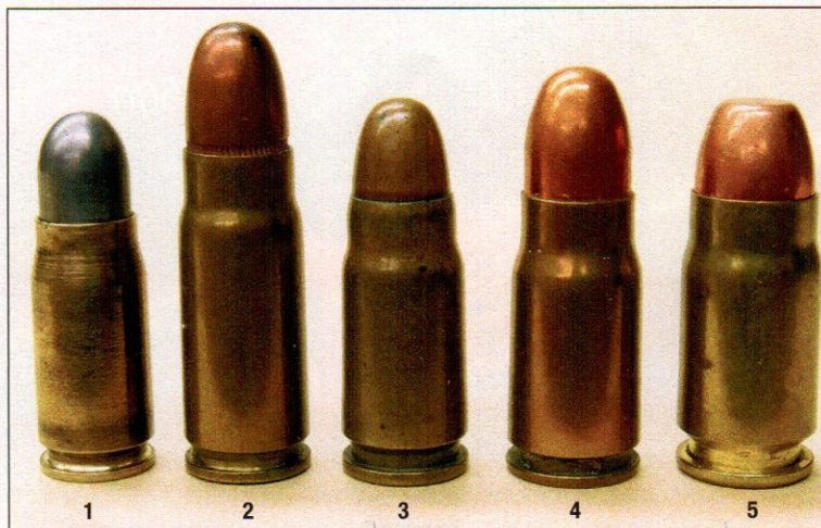
Bottleneck cartridges used in early automatics are the: (1) 7mm Japanese Nambu, (2) 7.63mm Mauser or 30 Mauser, (3) 7.65mm Parabellum or 30 Luger, (4) 8mm Japanese Nambu and today's (5) 357 SIG.
